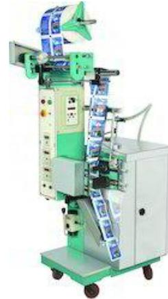
Fig 117: Fill-Seal Machine for Tomato Sauce
