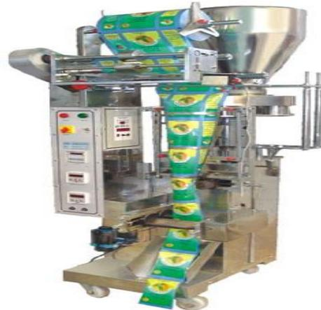
Fig 11: Automatic form fill seal machine
