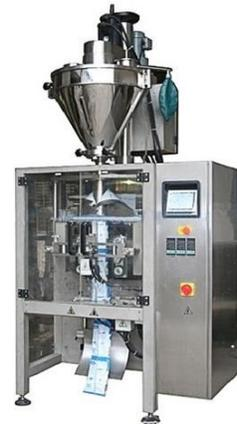
Fig 48: Form Fill-Seal Machine for Powder
