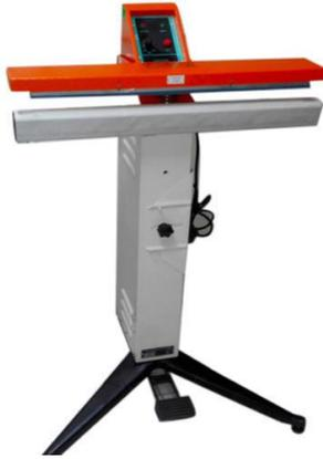
Fig 17: Pouch Sealing Machine
