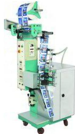
Fig 54: Fill-Seal Machine for Chili Sauce
